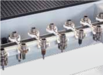
Upgrade to altogether 23 tool changing places possible (11 additionally)
