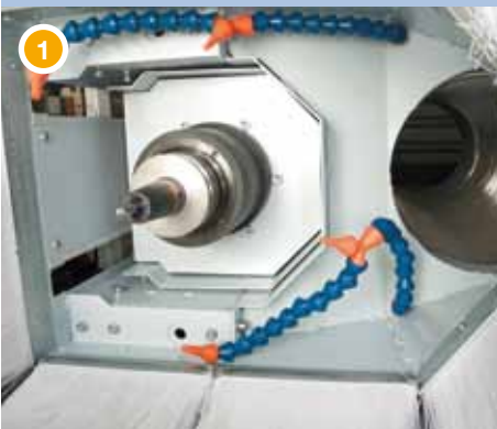
12 HP (9 kW) HSK routing spindle
