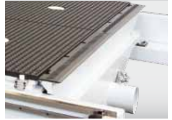
Extraction channel from below to clean the workpieces during exit of the boards
