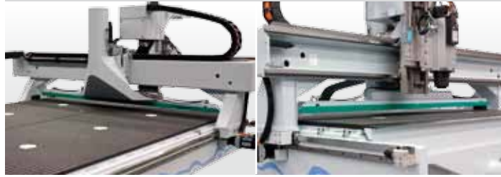
The complete Nest is pushed out (e.g. on a transport belt). The integrated dust extraction can carry out additional runs in order to clean the dummy board and workpieces.
