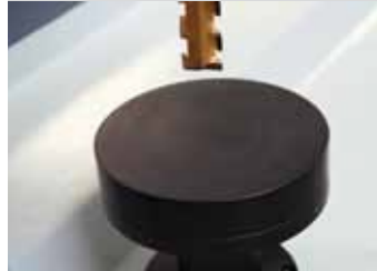
Following the tool change a tool length control is carried out and compared with the integrated tool data file
